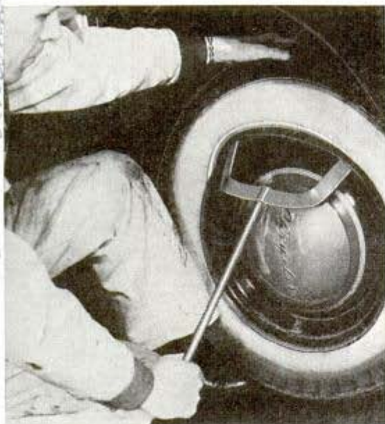
Tool pries tire at two points to avoid pinching tube
